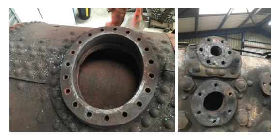
Photo (below left) shows progress on cutting out defective platework on the firebox backplate corners. Replacement formed material has been ordered for these corners. It also shows preparation for removal of lower wrapper section with stay and rivet removal and cutting of the firebox wrapper.
