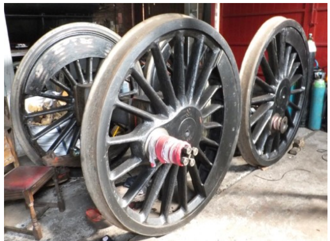
Progress at the end of June is seen here with rear axle primed (left) and centre plus front axle cleaned (right).
