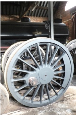
Progress at the end of June is seen here with rear axle primed (left) and centre plus front axle cleaned (right).
