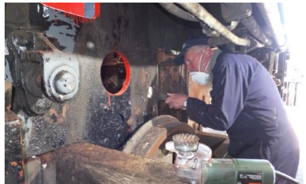
Tony Mayo and Glynn Pringle (right) have been removing old paintwork from the exterior surfaces of the frames.
