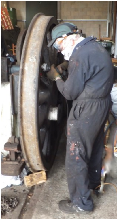
Fred Jones (left) is well on with the cleaning and painting of the driving axle wheel sets.
