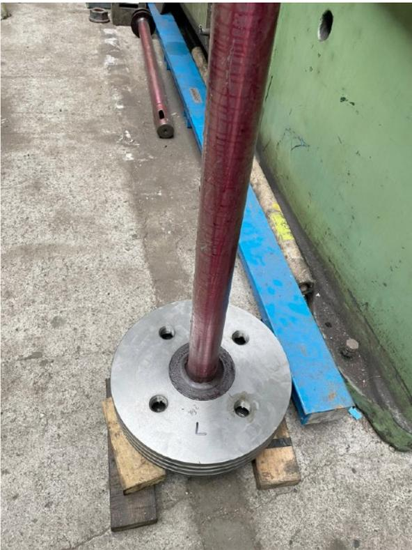
46441 Piston head machining, fitting of core plugs to the head and assembly to the piston rod is nearing completion and will hopefully be finished in early April. Photo (left) shows one partially completed assembly.
