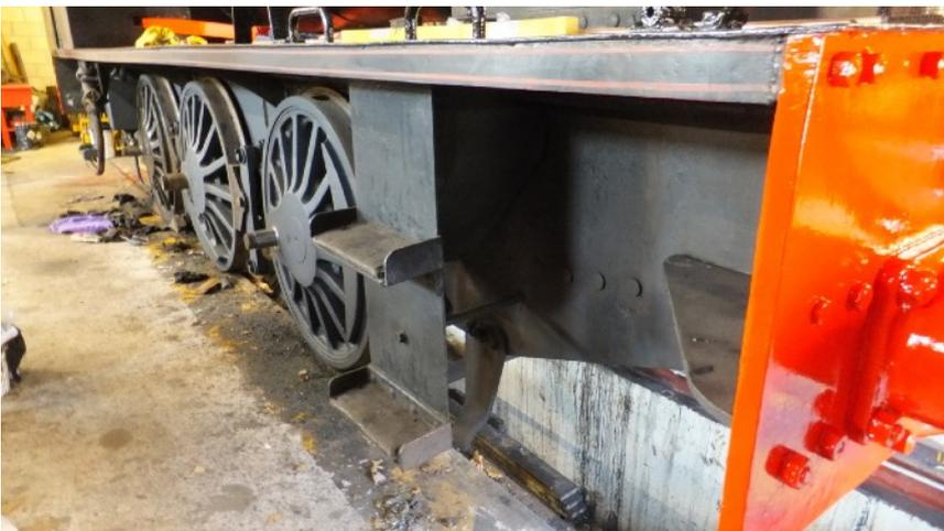
The opportunity has also been taken to give the loco a coat of paint below the running board and the photo (left) shows the frames and wheels now in undercoat.
