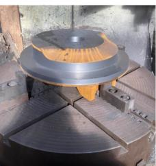
New piston rings are now machined and the photo (below left) shows the triple rings sat with one of the old double ring groove piston heads. Photo (below right) shows one of the new triple groove piston heads with core plugs now fitted.
