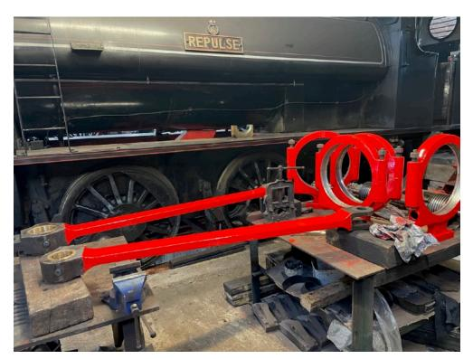
Re-assembly of the motion is progressing and the photo below shows the eccentric straps and coupling rods with a new coat of paint prior to assembly planned for the beginning of May.
