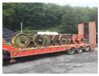
Several removed and spare Mk1 carriage wheel sets have been sent away for tyre turning. They can be seen here being loaded onto a trailer at Haverthwaite in mid September (Photo left).
