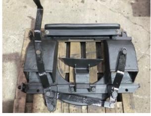
The stripped cleaned and repaired fire hole door assembly has been reassembled (photo left) and is ready for when it is needed for the boiler steam test.
