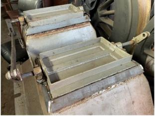
Four attempts at heating up the ejector exhaust ring to chimney joint were required before Chris Beet managed to split them. Photo (left) shows the items now separated.
