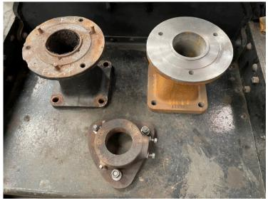
On the chassis, the new blast pipe and refurbished bast pipe cap are ready for assembly once new studs have arrived (photo left shows the cap with old and new blast pipe).
