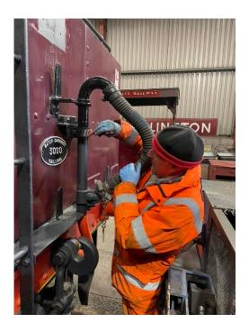
The lubrication system checks have been finished off including valve spindle oil feeds. New corks and oil box trimmings have been fitted, or refitted, where required (with just the cab area left to do).
