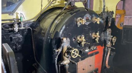
A new firebox concrete arch has been made. The footplate fittings have been reassembled and the footplate painting is underway (Photo left). The locomotive now looks complete but there are a range of minor jobs to finish before it can be steam tested. If work goes to schedule the insurance steam test should take place in the first half of June.
