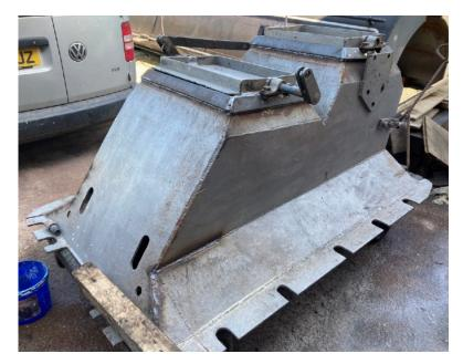
The Ivatt ashpan hopper stiffeners are now fully welded by Alistair Colquhoun as can be seen in the photo (left). It is ready to attach to the firebox once that has been steam tested out of the frames.
