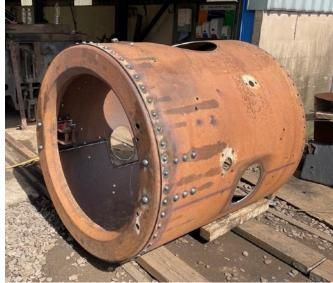
On the 10th May the smokebox was located onto the boiler (which had passed its hydraulic insurance test 5 days earlier). The assembly can be seen in the photo right and they were fully riveted together on the 11th.
