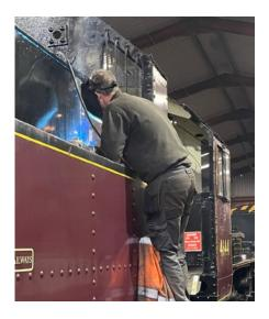
On the tender Alistair Colquhoun from John Fowler and Co. has fitted the newly fabricated water tank forward vents. Photos of the part finished task are shown here (left and right). These are now getting the required coats of paint.
