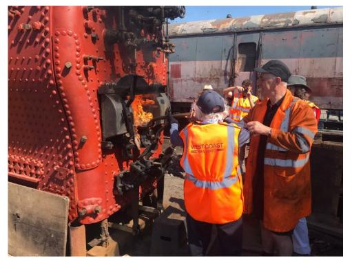
Through the next week the boiler was steamed several times at up to full pressure. There were only a few minor leaks that were readily rectified. The boiler insurance steam test was then scheduled and took place successfully on June 15th.
