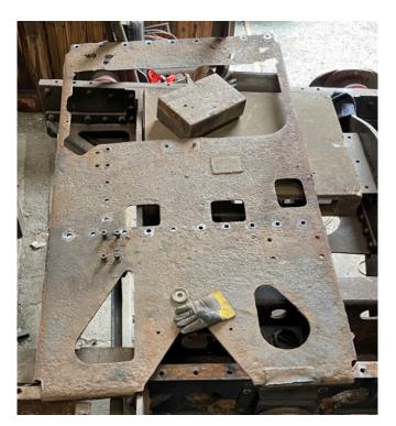
Removal of the horizontal rear stretcher first required dismantling the water scoop pivot bracket, which was in turn mounted to the water scoop vertical stretcher (pictured below). The top of the picture shows the underside of the horizontal rear stretcher. The rivet holes (top right) indicate where the pivot bracket had been mounted. The water scoop had been removed sometime during BR service.
