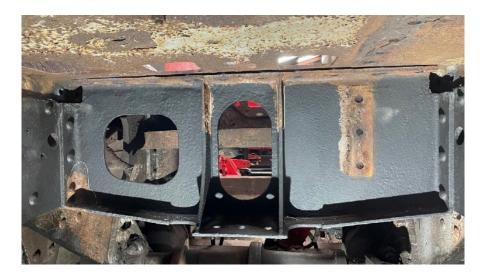
Removal of the horizontal stretcher has given us access to the steam brake stretcher fabrication which also needs repair by the John Fowler engineering team. This whole area between the frames can now be cleaned back to bare metal, primed and painted. Some further disassembly of components outside the frames is required to give access for the riveting gun (for when the new replacement horizontal stretcher is fitted).
