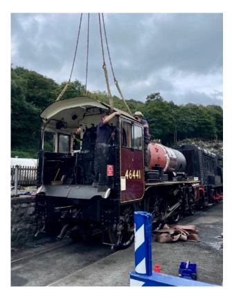
The cab roof was then lifted into position (photo left) and the damper and ashpan hopper door operating mechanism were fitted by the John Fowler engineering team.
