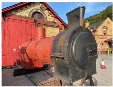
A fire was lit in the firebox on the 18th September and the boiler was checked over whilst in steam. The photo (left) was taken (in the rain) the day after - as evidenced by the soot marks around the firehole door.
