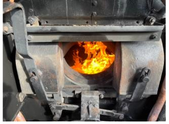
...and here we see the first warming fire. The loco was warmed through and by the end of the day sufficient steam pressure had been raised to test the injectors and check around for any other fittings that required nipping up. Time was taken to get some group photographs celebrating the loco in steam for the first time in 21 years.
