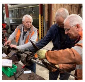
Chris Beet, Mike Hurst, Graham Magee and John McKay fitted the piston valves and checked the valve settings. The valve heads were measured and inserted into position (photo above right). By moving the loco with the diesel, the valve heads were confirmed as being to correct dimensions. The valves were then removed and rings fitted and contracted for re-insertion. This was straightforward to achieve given the experience of the team. The cotters were then fitted and the motion set-up finalised.
